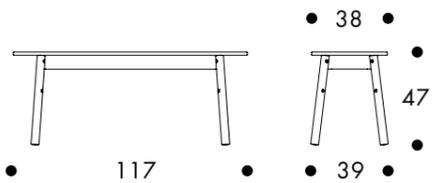
Solid ashwood legs, bent sheet steel structure, powder coated, benchtop with matt HPL surface and matt ABS edge banding, anti-slip glide.
