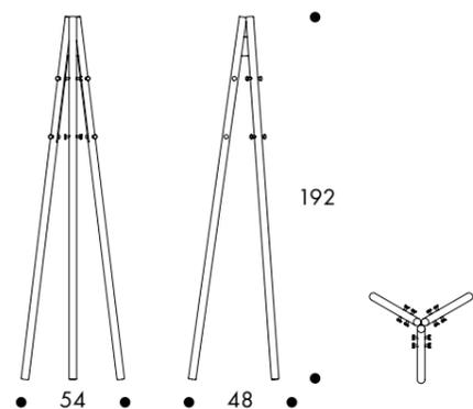
Three legs in solid ashwood, bent sheet steel structure, powder coated, twelve connector-hooks in dyed through polyamide, anti-slip glide.
