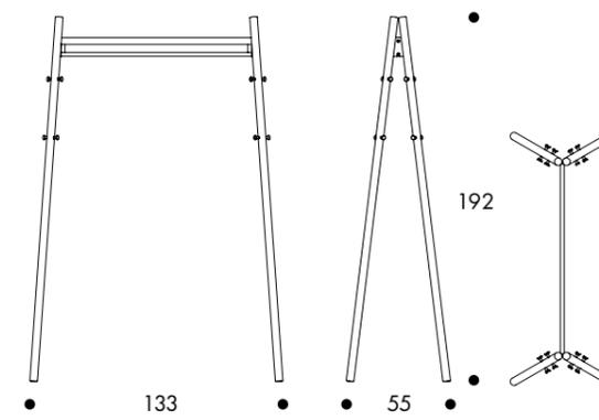
Four legs in solid ashwood, bent sheet steel structure and steel tubing, powder coated, sixteen connector-hooks in dyed through polyamide, anti-slip glide.
